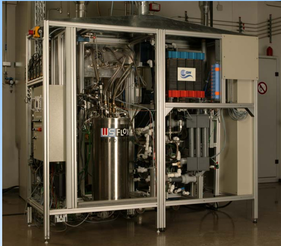
Prototype 1 (2004): 200 \times 70 \times 150 \text{ cm}^3 / 0.5 \text{ m}^3/\text{kW}_e
